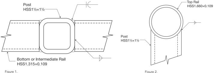
Connection of bottom or intermediate rail to post.
